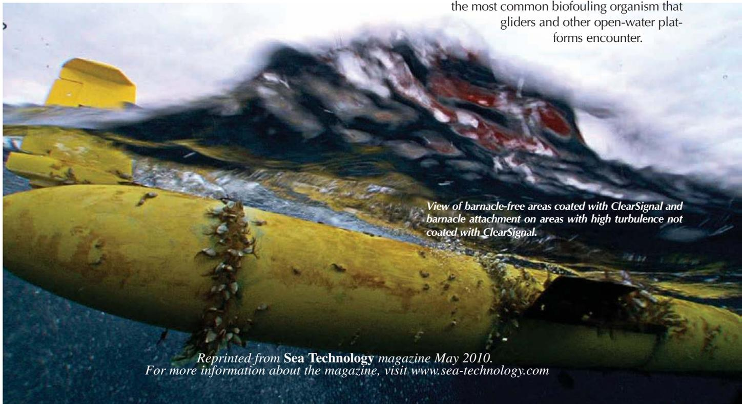
*View of barnacle-free areas coated with ClearSignal and barnacle attachment on areas with high turbulence not coated with ClearSignal.*
